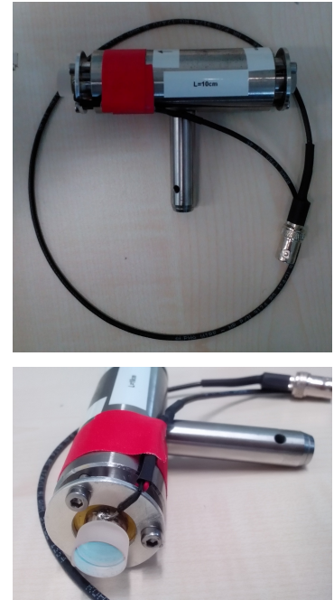
FIGURE 3.13: Pictures of self-made scanning Fabry-Pérot cavity. The cavity consists of a planar (left mirror in the top picture) and a concave mirror. While the last one was directly fixed to the casing the planar mirror was first glued onto a piezo and then attached to the tube as shown in the picture below. Further specifications are given in the text.
