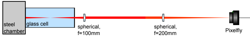
FIGURE 2.6: Schematic of the former optical setup for horizontal absorption imaging. While integrating the dimple beam into the experiment the previously used spherical f = 100 mm lens was replaced by the objective and a polarizing beamsplitter was inserted which allows for using the optical path for both the dimple beam and imaging (compare figure 2.5).
